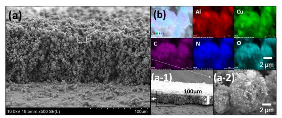
Figure 5. SEM images (a), elemental mapping (b) of Al/CuO microparticles produced by a typical electrospray process. (NC: 10 wt. %).
