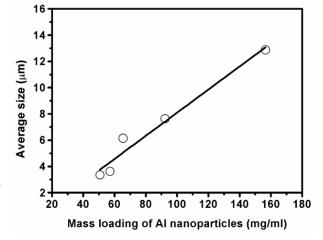
Figure 4. Average gelled particle size can be systematically increased by adding more nano-Al.
