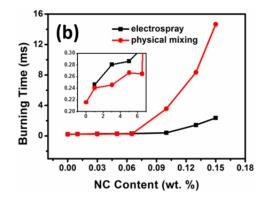
Figure 7. Pressure cell tests for thermite mixtures a) Maximum pressure; and (b) burning time of the nanothermite samples prepared by electrospray and physical mixing.
