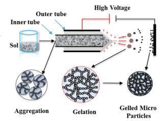
Figure 1. Schematic showing of electrospray formation of gelled microspheres.
