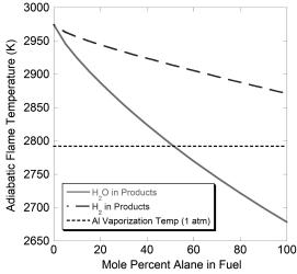
Fig. 3 Calculated adiabatic flame temperatures of  ${\rm CuO}{\rm -nAl-AlH_3}$  mixtures.
