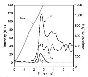
Fig. 8 Species profiles obtained in the T-jump TOF mass spectrometer for 25% AlH $_3$  fuel (balance is nanoaluminum)—CuO thermite.
