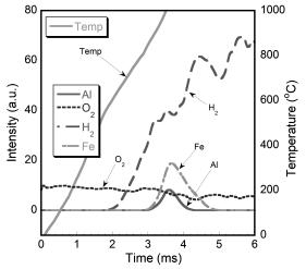
Fig. 12 Species profiles obtained in the *T*-jump TOF mass spectrometer for 25% AlH<sub>3</sub> fuel (balance is nanoaluminum)–Fe<sub>2</sub>O<sub>3</sub> thermite.
