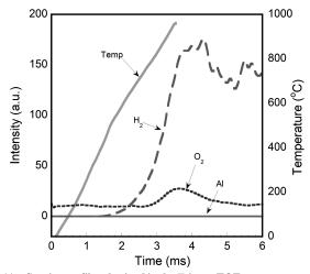
Fig. 11 Species profiles obtained in the T -jump TOF mass spectrometer for 100% AlH  $_3$  fuel—Fe  $_2{\rm O}_3$  thermite.
