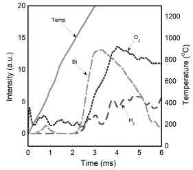
Fig. 10 Species profiles obtained in the T-jump TOF mass spectrometer for 25% AlH<sub>3</sub> fuel (balance is nanoaluminum)—Bi<sub>2</sub>O<sub>3</sub> thermite.
