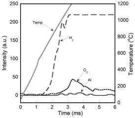
Fig. 7 Species profiles obtained in the T-jump TOF mass spectrometer for 100% AlH $_3$  fuel-CuO thermite.
