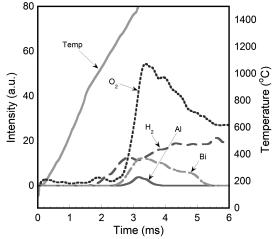
Fig. 9 Species profiles obtained in the T-jump TOF mass spectrometer for  $100\%~AlH_3~fuel-Bi_2O_3$  thermite.
