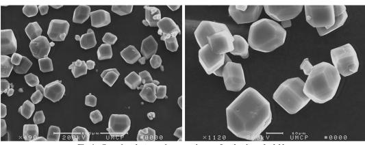
Fig. 1 Scanning electron microscopy image of  $\alpha$ -aluminum hydride.
