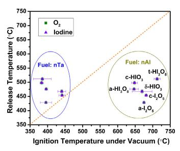
**Fig. 4.** I and  $O_2$  release temperature in neat iodine oxides/iodic acids, and the ignition temperature of corresponding nAl-based and nTa-based thermites under vacuum. Error bars correspond to at least two measurements. The orange dashed line stands for a perfect correlation. (For interpretation of the references to colour in this figure legend, the reader is referred to the web version of this article.)
