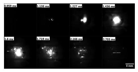
**Fig. 3.** Sequential snapshots of nTa/a-HI<sub>3</sub>O<sub>8</sub> thermite burning on a high rate heating  $(5 \times 10^5 \text{ °C/s})$  Pt wire under vacuum, captured by a high speed camera. The labels in each image are the time elapsed after triggering.
