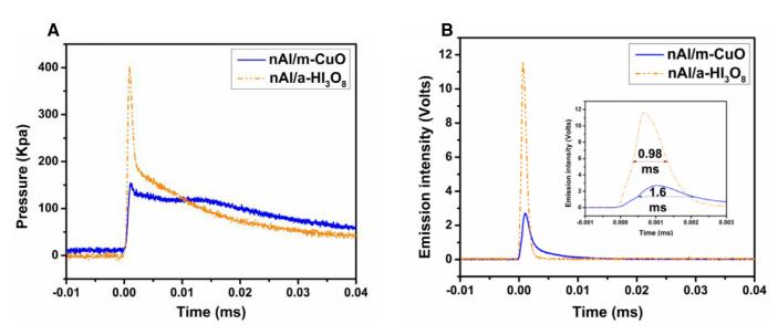
Fig. 5. Direct comparison between the pressure (A) and optical (B) trace of nAl/m-CuO and nAl/a-Hl<sub>3</sub>O<sub>8</sub>.
