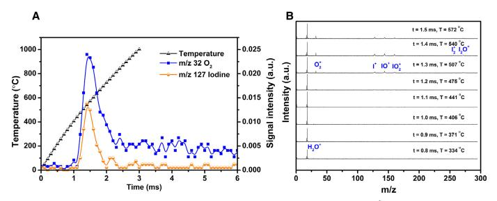
Fig. 1. Representative plot showing the temporal profile of oxygen and iodine upon heating  $a-HI_3O_8$  when heated at  $\sim 5 \times 10^5$  °C/s (A); time-resolved mass spectra of  $a-HI_3O_8$  (B).
