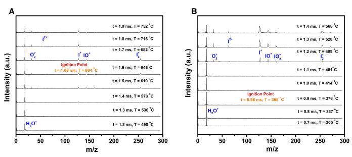
Fig. 2. Time-resolved mass spectra of nAl/a-HI<sub>3</sub>O<sub>8</sub> (A) and nTa/a-HI<sub>3</sub>O<sub>8</sub> (B).
