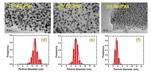
Fig. 2 (a), (b), (c) Formation of Ag, Cu, and Ni within the PVA matrix by the LPSW technique. Insets show selected area diffraction patterns for each sMNPs-PVA film. (d), (e), (f) Particle size distributions of Ag, Cu, and Ni respectively in PVA films (from a, b, c respectively). These films were coated on a 0.2 mm glass substrate.
