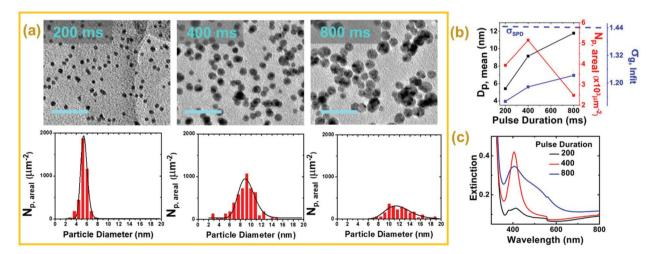
Fig. 6 (a) TEM images (scale bar: 50 nm) and the corresponding PSDs of Ag sMNPs-9k PVA films fabricated for different pulse durations for a laser energy flux of 20 W cm<sup>-2</sup>, (b) effect of pulse duration on the mean particle diameter, geometric standard deviation ( $\sigma_g$ ), and areal mass density in 9k PVA films, (c) extinction spectra of Ag sMNPs-PVA films fabricated by LPSW for different number of pulses. Substrate used is a 1 mm glass slide.
