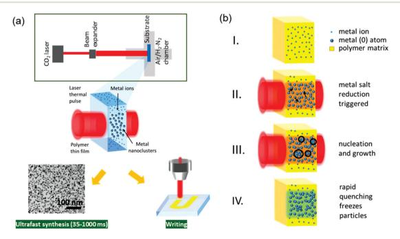
Fig. 1 (a) Schematic showing the laser photothermal synthesis and writing (LPSW) to form small metal nanoclusters directly in the polymer thin film. (b) Basic mechanism of nanocluster formation by LPSW.
