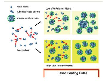
Fig. 7 Primary growth mechanisms in LPSW of metal particles in polymer matrices with different molecular masses, resulting in two different kinds of size distributions.
